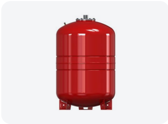
Onyx Onyx 100LHEATING 100L Red Heating Expansion Vessel 1" 1.5 Bar | Genuine Replacement Spare Part SKU EDDONYX09 MPN 100LHEATING
