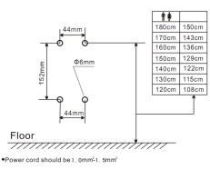
The power cord Supplying the hand dryer should be at least 1.5m<sup>2</sup> 2 Core & Earth
