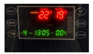
Press ON/OFF button to turn boiler on – Standby
