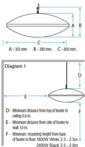
The Herschel PULSAR must be located in a position to allow proper and efficient use but one that ensures hot parts are not touched accidentally. The recommended installation height of the White 1800W Pulsar is 2.3m - 2.5m (90" - 110") from the floor.
