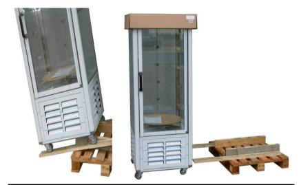
Roll the display gently over the planks. Hold back the display as soon as the planks start to tilt.
