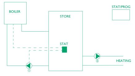
Pump away from the store The cylinder thermostat switches the boiler and pump ① The room stat/programmer switches the heating pump ②
