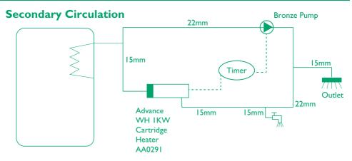
Set the WHI at 45°C to maintain temperature in the secondary loop without affecting the store temperature, costing just pennies per day.
