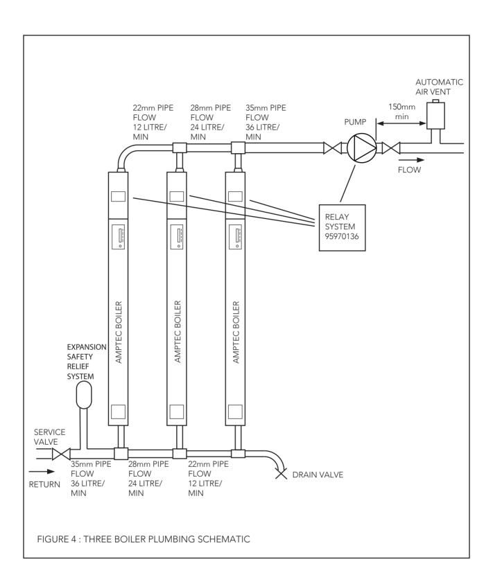
A typical plumbing schematic connecting 3 x 1200 boilers together.
