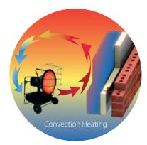
Conventional Convection Heating only heats the air within the building so the inner wall absorbs none of the heat being produced. This in turn means the walls are acting as 'cold radiators' which then very rapidly cool the air within the room once the heating system stops working.
