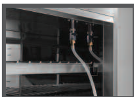
Internal tap with tube for easy draining
