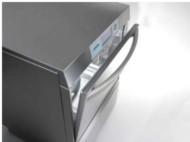
Do not close the machine door fully so that the inside of the machine can dry better. A special latch position in the door clasp is provided for this purpose. This is also important for long-term corrosion protection, even for stainless steel.
