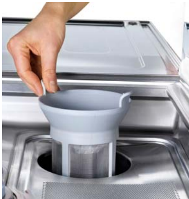
Remove the filter cylinder
